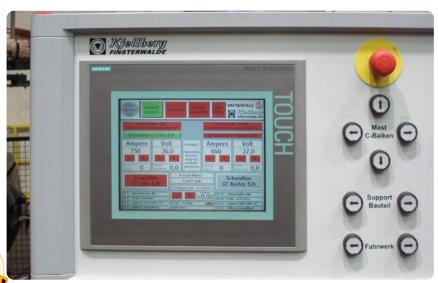
The centrepiece of the electrotechnical renewal is the central control panel for controlling the mechanical components and the welding process
