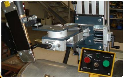
Detail: The manual positioning in X and Y direction is still possible as well as the height correction via manual control panel
