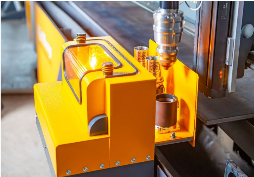
Caption: The Q-Torch Auto Change System paves the way for automated plasma cutting. (© Photo: Kjellberg Finsterwalde)
