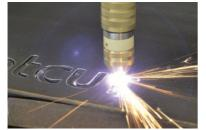
Picture: Kjellberg-SilentCut.jpeg - Cutting of mild steel with reduced the sound pressure level with Silent Cut
