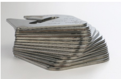
Picture 1: Metallic blank cut surfaces with the HiFinox technology for plasma cutting of stainless steel and aluminium (© Photo: Kjellberg Finsterwalde)
