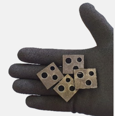
Plasma cutting of small holes
