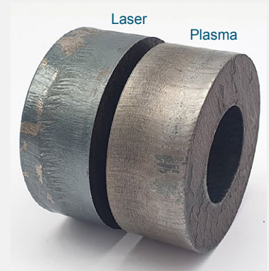
Comparison of cut surfaces 25 mm mild steel
