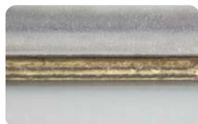
Perfect seam surface even in case of coated surfaces, v = 3 \text{ m/min}
