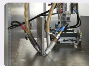
Modified mounting of the hinged arms
