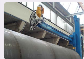
System solution: Welding mast with KA 2-UPP for longitudinal welding on tubes
