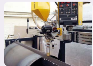
KA 2-UP for longitudinal welding with backing bar
