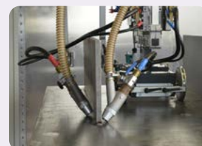
Modified mounting of the hinged arms
