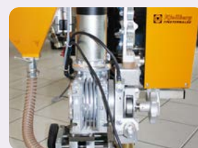
Robust feeding gear for wire up to Ø 5.0 mm
