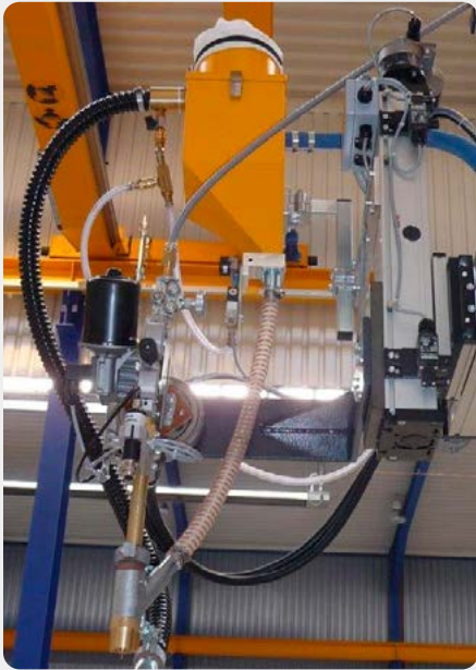
Flux container 10 l with pressure and suction hose
