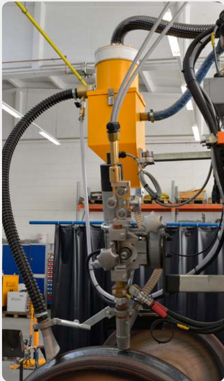
Flux system 6 l with manual flux shutoff device, sieve and feed hose
