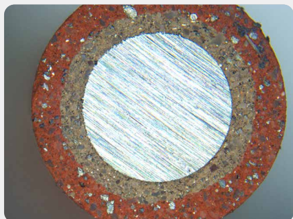
Basic coating outside, rutile cover inside
