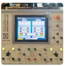
Before - after: A welding database is now an integral part of the control system. The welder reproduces the welding results at the push of a button, thus ensuring a consistent quality.
