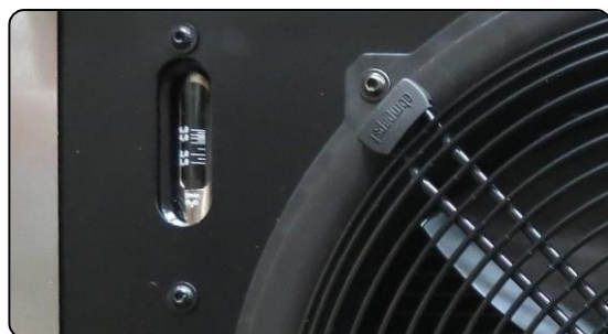
Cooler C3 with rotary vane pump, float display 1-6l/min, magnet switch, potential free on terminal .17.400.151.3
