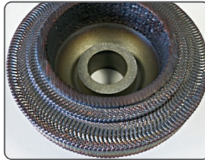
Example: fitting made from 1.4404, Ø 190 mm, 17 kg
