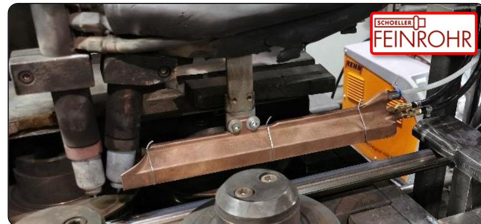
Measurement O 2 concentration also during welding
