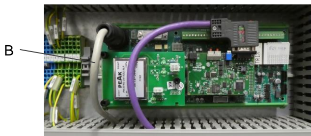
Interface for installation in control cabinet (top-hat rail)
