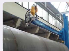
System solution: Welding mast with KA 2-UPP for longitudinal welding on tubes
