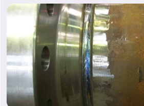
Tube-flange connection welded with manual SAW equipment
